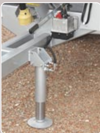
21 Pie hidráulico Hydraulic parking jack
