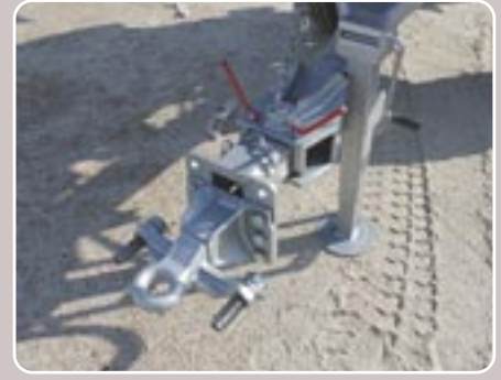
15 Lanza giratoria articulada Articulated draw-bar
