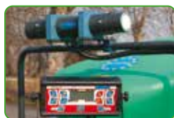
Interceptor sonar com eletroválvula e monitor
